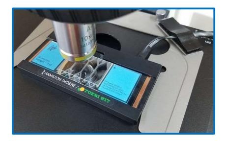
The MiniTherm Plus consists of a digital controller and a glass microplate that fits between standard microscope stage clamps.
